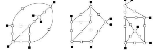
Fig. 7. Possible topologies for a (6, 6) ETS in a left-regular graph with  $d_l = 4$  and g = 6: topologies with only one variable node connected to two unsatisfied check nodes.
