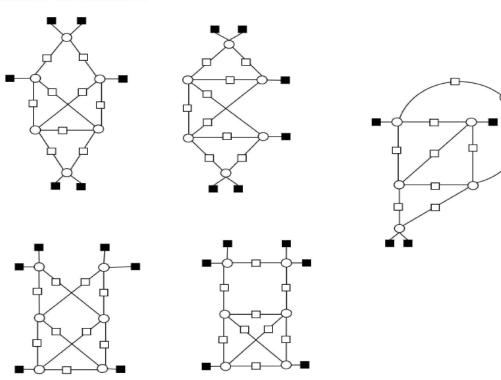
Fig. 8. Possible topologies for a (6, 6) ETS in a left-regular graph with  $d_l = 4$  and g = 6: topologies with only two variable nodes connected to two unsatisfied check nodes.
