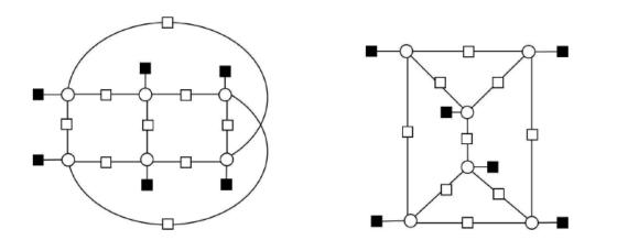
Fig. 6. Possible topologies for a (6, 6) ETS in a left-regular graph with  $d_l = 4$  and g = 6: the only two possible absorbing set topologies.
